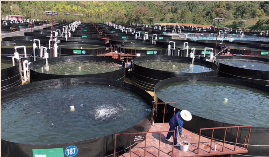
Modular land-based recirculating aquaculture system of CIMC Intelligent
