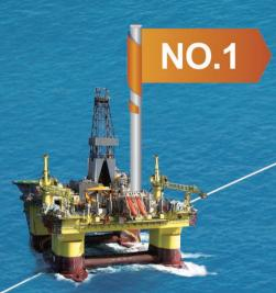
COSL "Pioneer", delivered in October 2010, is the first deep-water semi-submersible drilling platform delivered by China. It started being applied in the Norwegian North Sea operation from 2011 and was awarded "Rig of the Month" of Norwegian North Sea for 3 times.
