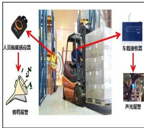
Case of Forklift Anti-collision Improvement
