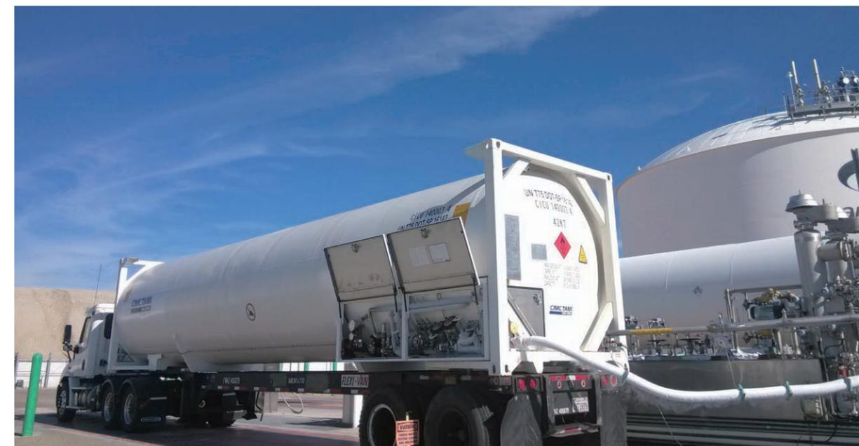
may contract for LNG tank containers for dangerous cargos of Class 2.1 (LNG belongs to the dangerous goods of Class 2.1) which may be shipped under the international standards of IMDG/ADR/RID/TC/CSC, and the products may arrive at and depart from the ports just through the wharf for the common containers of dangerous cargo.
